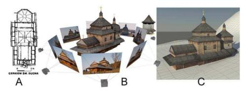
Fig. 1. Technical projection and photography scheme: A – technical projection of the church; B – scheme of photographing from the outside of current church; C – view of the church before 1736
