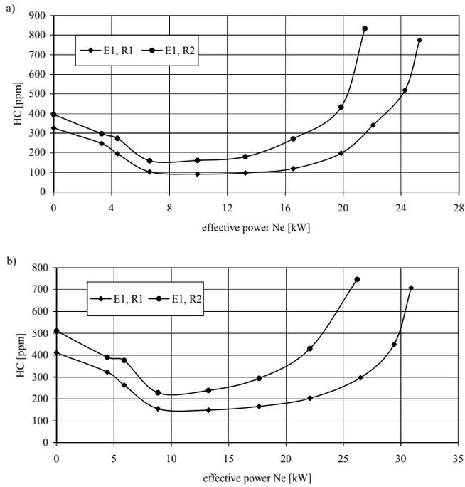
Fig. 3. Variation of HC emission level in exhaust gases in function of effective power ( $N_e$ ) of tractor's engine S-4003 depending on injector's spray nozzle tips wear level: a) 1500 rpm, b) 2000 rpm; E1 – pressing sections 0% of wear, R1 – spray nozzles 0% of wear, R2 – spray nozzles 100% of wear
