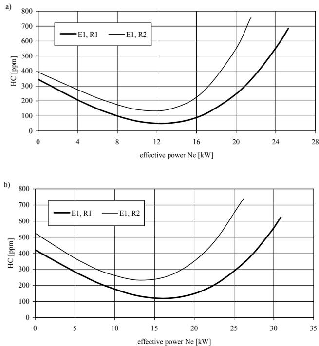
Fig. 5. Variation of HC emission level in exhaust gases in function of effective power ( $N_e$ ) of tractor's engine S-4003 depending on injector's spray nozzle tips wear level (regression analysis): a) 1500 rpm, b) 2000 rpm; E1 – pressing sections 0% of wear, R1 – spray nozzles 0% of wear, R2 – spray nozzles 100% of wear
