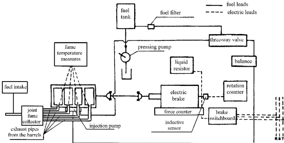
Fig. 1. The diagram of the test stand
