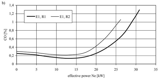
Fig. 4. Variation of CO emission level in exhaust gases in function of effective power ( $N_e$ ) of tractor's engine S-4003 depending on injector's spray nozzle tips wear level (regression analysis): a) 1500 rpm, b) 2000 rpm; E1 – pressing sections 0% of wear, R1 – spray nozzles 0% of wear, R2 – spray nozzles 100% of wear
