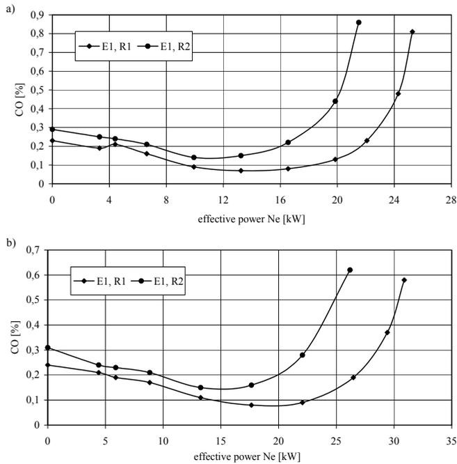
Fig. 2. Variation of CO emission level in exhaust gases in function of effective power ( $N_e$ ) of tractor’s engine S-4003 depending on injector’s spray nozzle tips wear level: a) 1500 rpm, b) 2000 rpm; E1 – pressing sections 0% of wear, R1 – spray nozzles 0% of wear, R2 – spray nozzles 100% of wear
