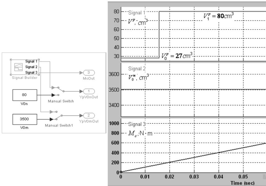
Fig. 7. The internal structure of “variable managements” block
