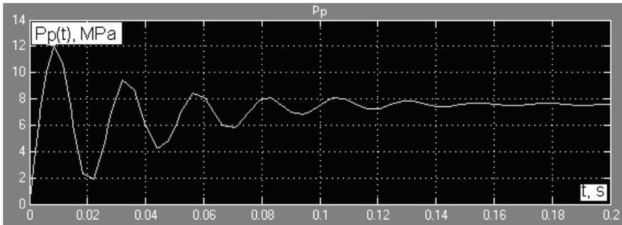
Fig. 8. Results of numerical simulation of dynamics  $\bar{p}_p(t)$ :  $V_0^p = 80\text{cm}^3$ ;  $t_0^p = 0\text{s}$
