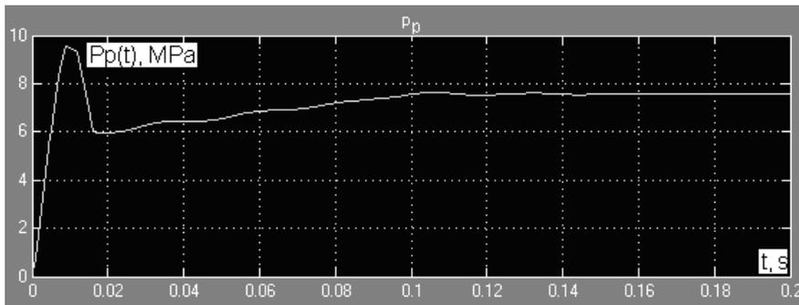
Fig. 9. Results of numerical simulation of dynamics  $\bar{p}_p(t)$ :  $V_0^p = 27\text{cm}^3$ ;  $t_0^p = 0,016\text{s}$
