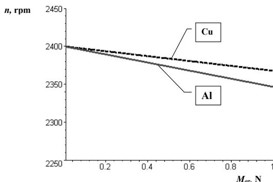
Fig. 6. Dependence  $n=f(M_{or})$  for copper and aluminium RWB
