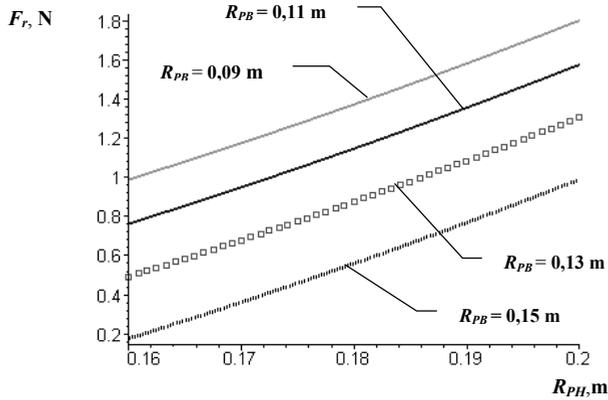
Fig. 2. Dependence  $F_r = f(R_{PH})$  for RWB with different  $R_{PB}$
