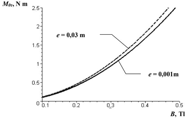
Fig. 5. Dependences  $M_{0r} = f(B)$  with maximal and minimal  $e$
