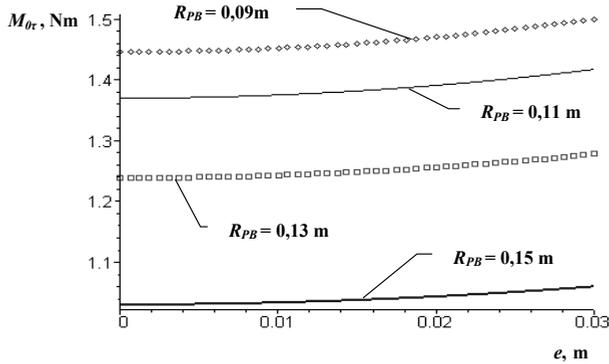
Fig. 3. Dependences  $M_{0r} = f(e)$  for RWB with different inner radius
