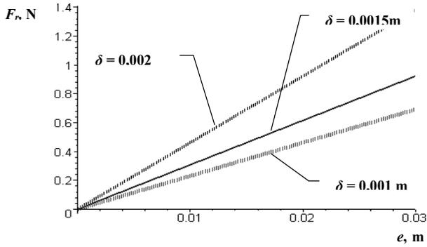
Fig. 4. Dependence  $F_r = f(e)$  for RWB of different thickness
