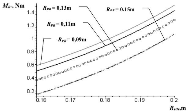
Fig. 1. Dependence  $M_{or} = f(R_{pH})$  for RWB with different  $R_{pB}$
