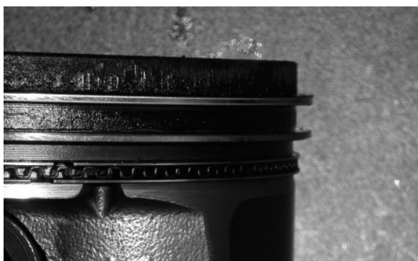
Fig. 3. Visual evaluation of the technical condition of piston rings and the piston ring area in the engine fuelled by hydrocarbon gasoline with 5%(v/v) ethanol additive
