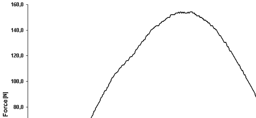
Fig. 4. Exemplary force-response curve recorded at the first impact from 70 mm height, apple after storage
