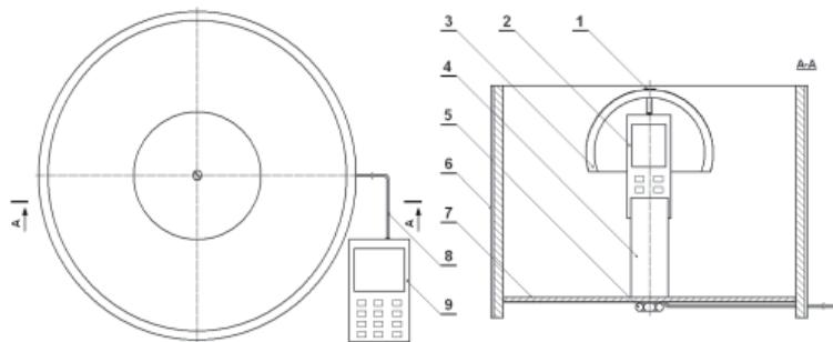
Fig. 1. Rainfall water parameter indicator developed at the Western Pomeranian Research Centre of the Institute for Land Reclamation and Grassland Farming in Szczecin: 1-top screw joint, 2-dynamometer, 3-hollow hemisphere, 4-dynamometer cantilever, 5-bottom screw-joint, 6-cylinder, 7-cylinder bottom, 8-LV conductors, 9-measuring data recorder
