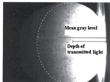
Parameters determined on the base of transmitted light system.
