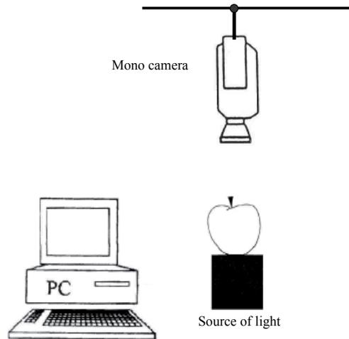
Setup of transmitted light system.
