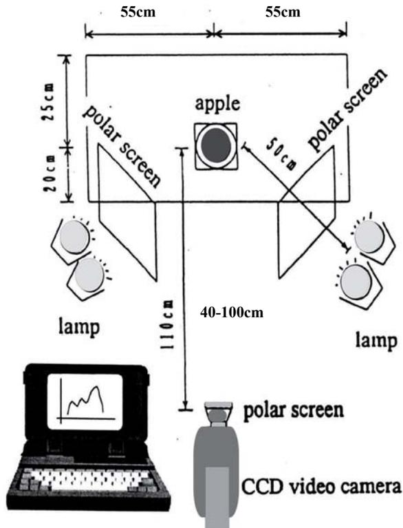
Fig. 1. Machine vision system
