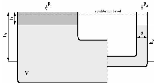
Fig. 2. Physical model of the object of study:  $h_1$  – open tank water column height considered;  $h_2$  – assumed height of water column entering the intake chamber at constant conical turbine operation parameters;  $p_1$  – water surface pressure in the open tank;  $p_2$  – water surface pressure in the intake chamber;  $d$  – water stream diameter in the intake chamber;  $V$  – volume of hypolimnetic water to be treated by pulverising aeration
