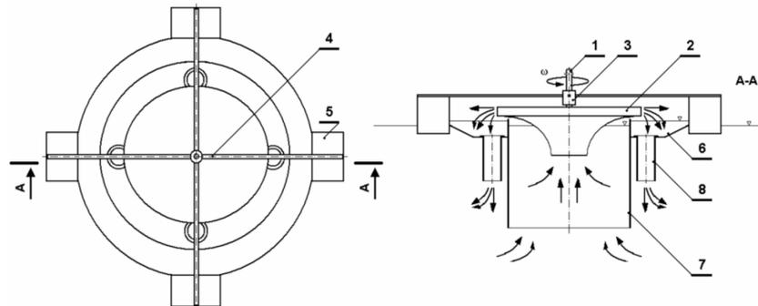
Fig. 1. Pulverising aerator developed at Institute for Land Reclamation and Grassland Farming (ILRGF) Western Pomeranian Research Centre in Szczecin: 1 – propeller shaft; 2 – conical turbine; 3 – hub; 4 – support; 5 – float; 6 – aeration chamber; 7 – water intake chamber; 8 – drain pipe
