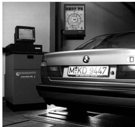
Fig. 4. The diagnostic line SCREEN-TESTLINE 7000 supplied by BEISSBARTH [ www.precyzja.pl ]
