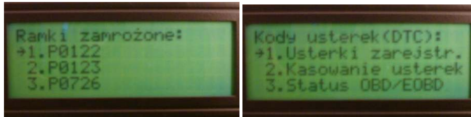
Fig. 7. The exemplary parameters during the system operation in MODE 2 and 3 (registered errors) P0122 – low signal of the level sensor of throttle position TP, strategy: urgency characteristics A, the lamp MIL lights, P0123 – high signal of the level sensor of throttle position TP, strategy: urgency characteristics B, the lamp MIL lights, P0726 – motor velocity inlet circuit RPM – signal beyond the range, strategy: RPM = 8500 rpm, the lamp MIL lights
