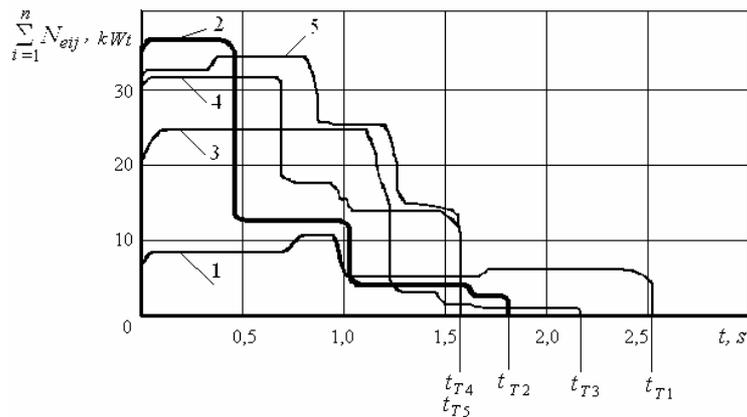
Fig. 3. Diagram of IR engines power consumption by execution of the certain trajectory
