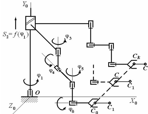
Fig. 2. Structural-kinematics model of the IR type SCARA
