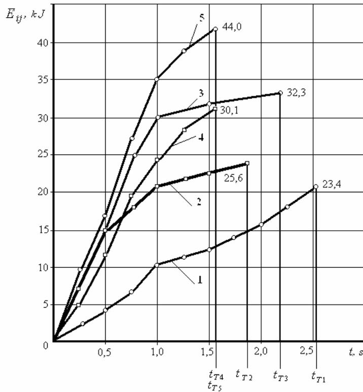
Fig. 4. Diagram of IR energy consumption by an execution of a certain trajectory
