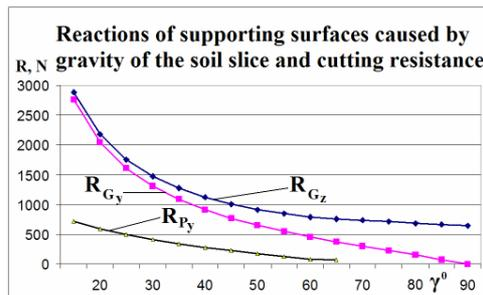
Fig. 6. Reactions of the lower and lateral supporting surfaces caused by gravity of the soil slice and share cutting resistance depending on the inclination angle  $\gamma$  of the horizontal generatrix
