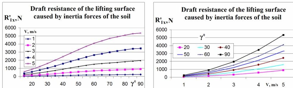
Fig. 3. Draft resistance of the lifting surface caused by the soil inertia forces of the soil slice depending on speed  $v$  and the inclination angle  $\gamma$  of the horizontal generatrix
