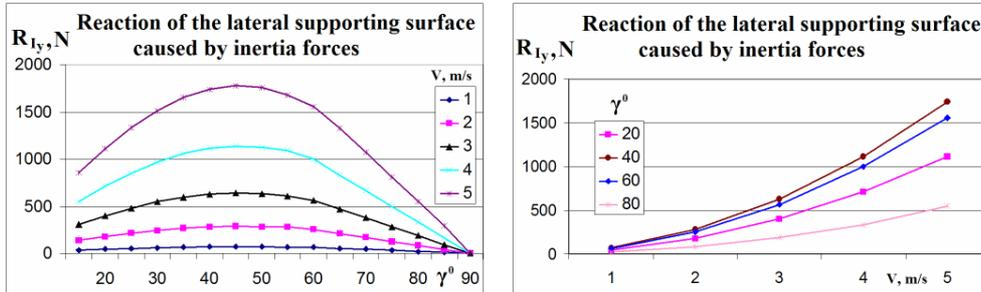
Fig. 8. Reaction of the lateral supporting surfaces caused by soil inertia forces depending on speed  $v$  and the inclination angle  $\gamma$  of the horizontal generatrix
