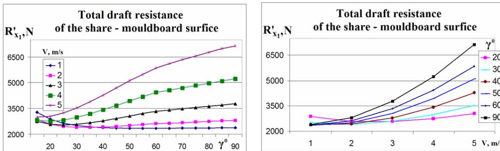
Fig. 9. Total draft resistance of the share-mouldboard surface caused by soil gravity, inertia forces, adhesion and share cutting resistance depending on speed  $v$  and the inclination angle  $\gamma$  of the horizontal generatrix
