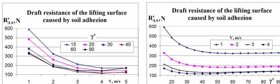
Fig. 4. Draft resistance of the lifting surface caused by soil adhesion depending on speed  $v$  and the inclination angle  $\gamma$  of the horizontal generatrix
