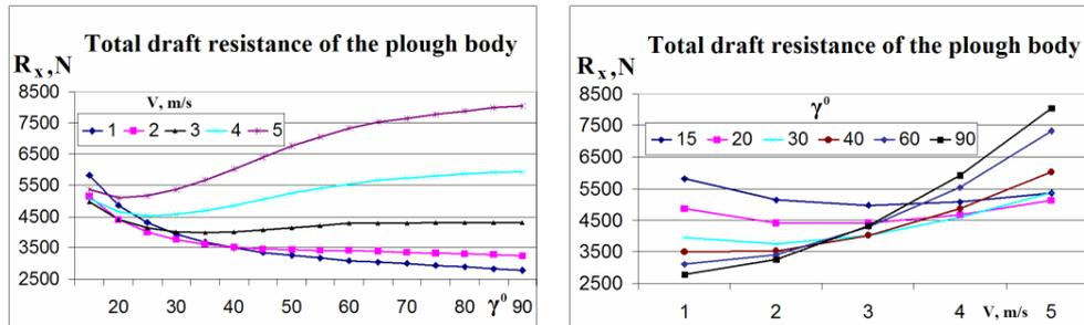
Fig. 11. Total draft resistance of plough body depending on speed  $v$  and the inclination angle  $\gamma$  of the horizontal generatrix
