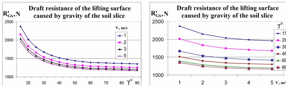
Fig. 2. Draft resistance of the lifting surface caused by the gravity of the soil slice depending on speed  $v$  and the inclination angle  $\gamma$  of the horizontal generatrix
