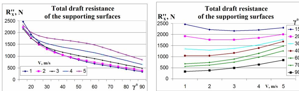
Fig. 10. Total draft resistance of the supporting surfaces depending on the speed  $v$  and the inclination angle  $\gamma$  of the horizontal generatrix
