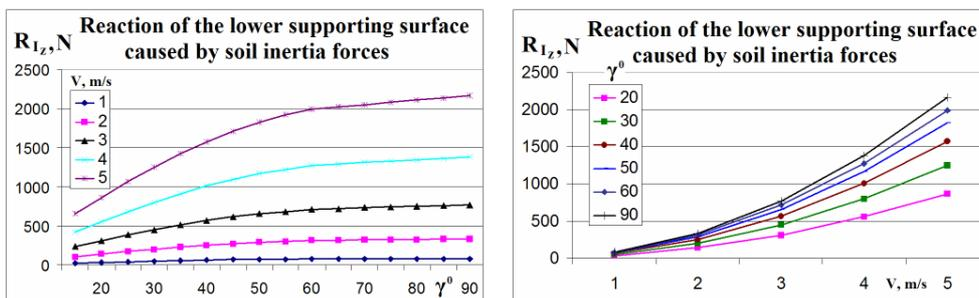
Fig. 7. Reaction of the lower supporting surface caused by soil inertia forces depending on speed  $v$  and the inclination angle  $\gamma$  of the horizontal generatrix.
