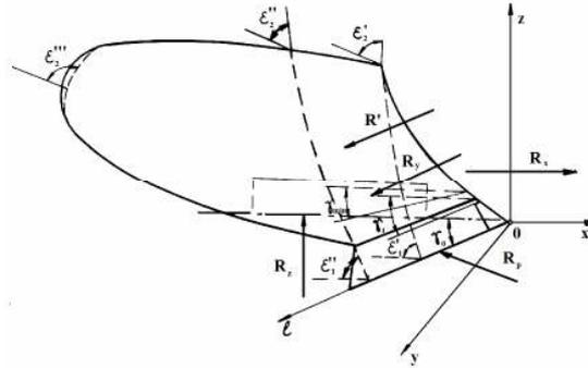
Fig. 1. A scheme of a plough body, its parameters and acting forces
