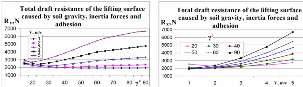
Fig. 5. Total draft resistance of the lifting surface caused by soil gravity, inertia forces and adhesion depending on speed  $v$  and the inclination angle  $\gamma$  of the horizontal generatrix
