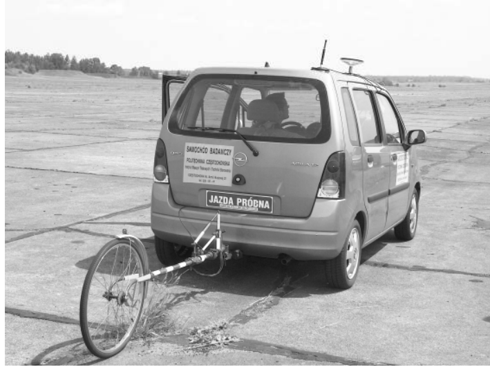
Fig. 2. One of the testing vehicles during road surveys made with the GPS system and the „fifth wheel”, respectively
