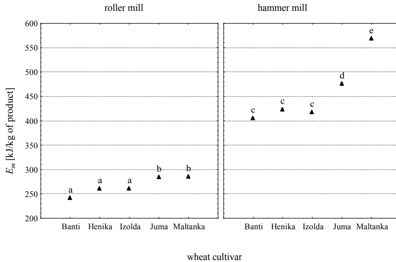
Fig. 3. The grinding efficiency index of wheat cultivars obtained for a roller mill and a hammer mill
