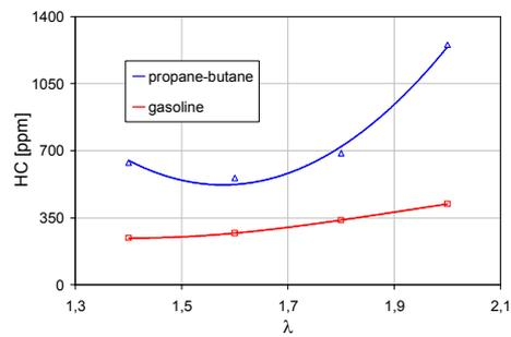
Fig. 18. Hydrocarbons emission of an engine with gas and liquid supply system
