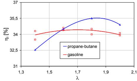
Fig. 14. Indicated efficiency of an engine with gas and liquid supply system for  $Q_{in}/Q_{tot} = 2.5\%$
