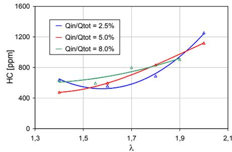
Fig. 10. Hydrocarbons emission of gas engine
