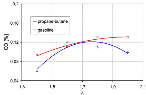
Fig. 20. Carbon monoxide emission of an engine with gas and liquid supply system
