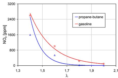
Fig. 17. Nitric oxide emission of an engine with gas and liquid supply system
