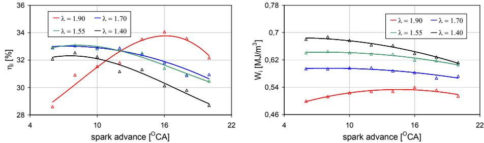
Fig. 5. Effect of ignition advance angle on indicated efficiency and indicated work of a gas engine for  $Q_{in}/Q_{tot} = 8.0\%$
