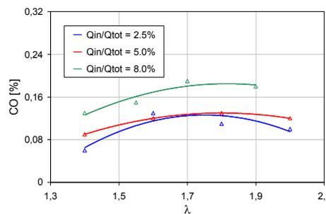
Fig. 12. Carbon monoxide emission of gas engine
