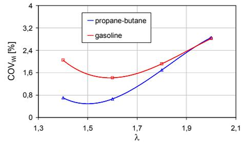
Fig. 16.  $COV_{wi}$  factor indicated work of an engine with gas and liquid supply system for  $Q_{in}/Q_{tot} = 2.5\%$
