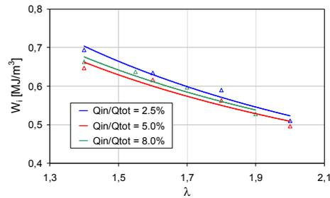
Fig. 6. Indicated work of 97 cycles of gas engine operation
