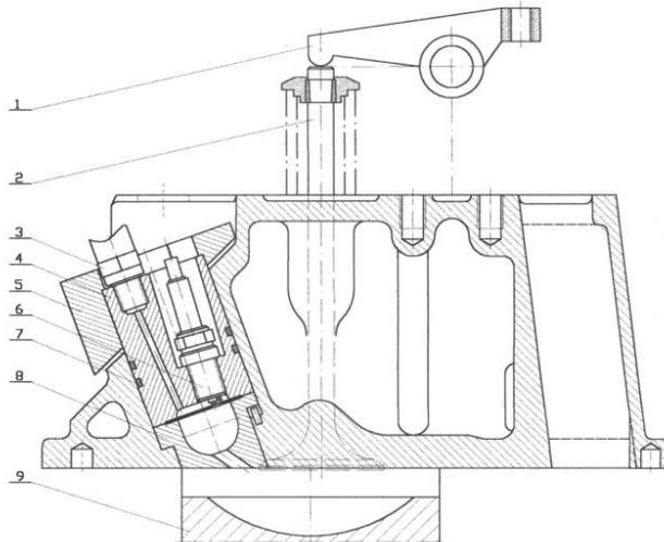
Fig. 1. Test engine head with prechamber: 1 – valve rocker, 2 – inlet valve, 3 – flame suppressor, 4 – prechamber body, 5 – retaining cover, 6 – spark plug, 7 – sealing ring, 8 – prechamber, 9 – piston
