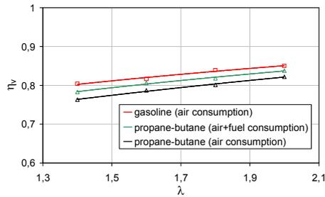
Fig. 15. Volumetric efficiency of an engine with gas and liquid supply system for  $Q_{in}/Q_{tot} = 2.5\%$
