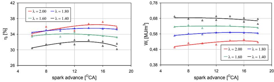
Fig. 3. Effect of ignition advance angle on indicated efficiency and indicated work of a gas engine for  $Q_{in}/Q_{tot} = 2.5\%$
