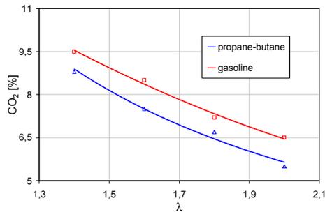
Fig. 19. Carbon dioxide emission of an engine with gas and liquid supply system
