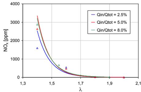
Fig. 9. Nitric oxide emission of gas engine
