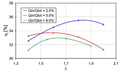
Fig. 7. Indicated efficiency of gas engine
