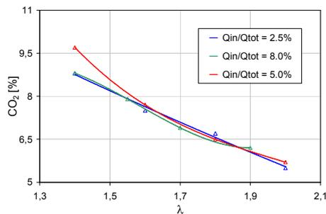
Fig. 11. Carbon dioxide emission of gas engine
