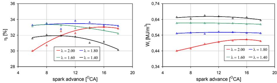
Fig. 4. Effect of ignition advance angle on indicated efficiency and indicated work of a gas engine for  $Q_{in}/Q_{tot} = 5.0\%$
