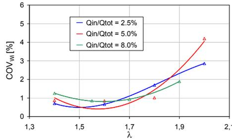
Fig. 8.  $COV_{w_i}$  factor indicated work of 97 cycles of gas engine operation
