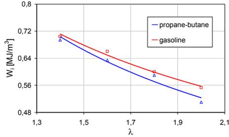
Fig. 13. Indicated work of an engine with gas and liquid supply system for  $Q_{in}/Q_{tot} = 2.5\%$
