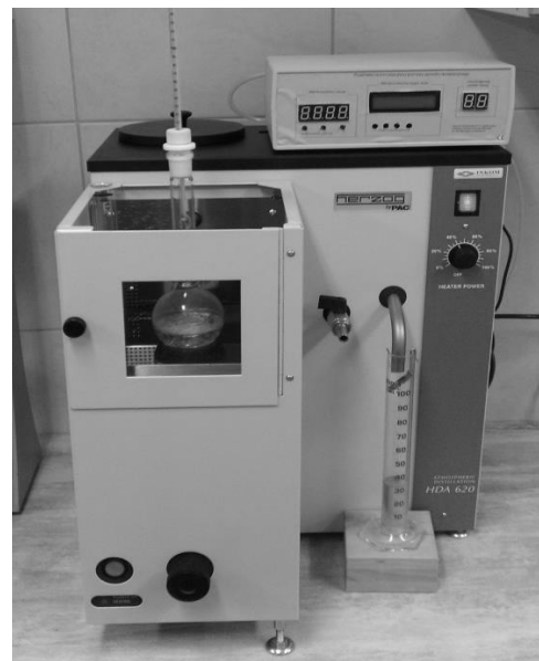
Fig. 3. Photo bench equipped with a distiller HAD 620/1 by Herzog
