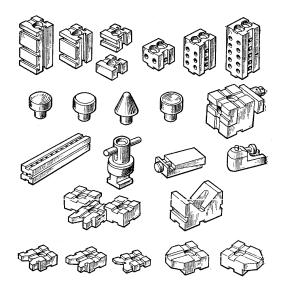
Fig. 3. Elements universal modular system UMA machine tool adaptations
