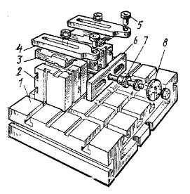
**Fig. 4.** Scheme build prefabricated universal machine tool accessories: 1 – square plate, 2 – rectangular pillar, 3 – support,
