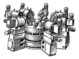
Fig. 2. Assembly quicky adjustable with drum machines revolving heads and rotary table
