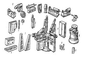
**Fig. 1**. Scheme of separation metal-cutting machine into individual interchangeable units: 1 - ground, 2 - axle, 3 - shoes, 4 - intermediate plate, 5 - nozzles, 6 - power head, 7 - tilting brackets, 8 - electrical cabinet, 9 - filter for oil tank, 10 - pitch table, 11 - benchboard
