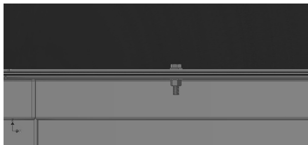
Fig. 13. Generated screw connection of the ring holding down the membranes and the angle section at the top of the tank [own elaboration]
