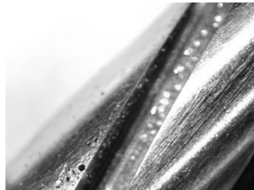
Fig. 5. A seized component of the plunger and barrel assembly of a fuel injector's needle
