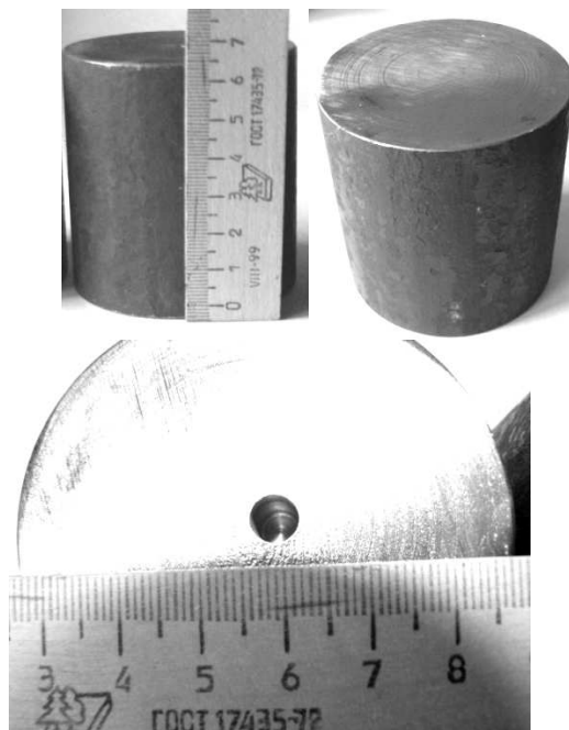
Fig. 1. The steel sample with an artificial reflector - drilling with a flat bottom: a - general view of the sample, b - a flat surface scanning with an ultrasound transducer, c - the flat surface of the sample with a flat bottom made by the drilling
