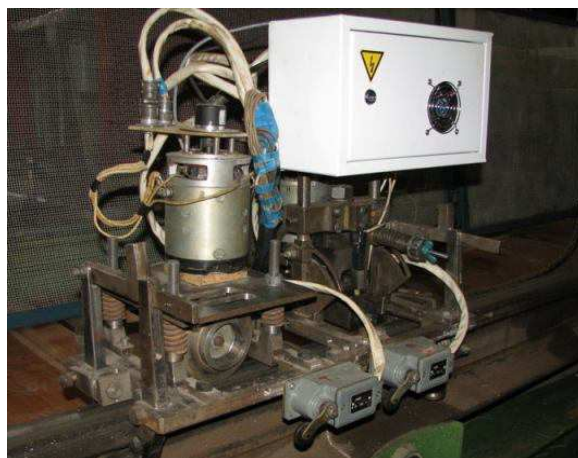
Fig. 1. Stand «Friction machine for studying frictional properties of the contact of wheel-rail»
