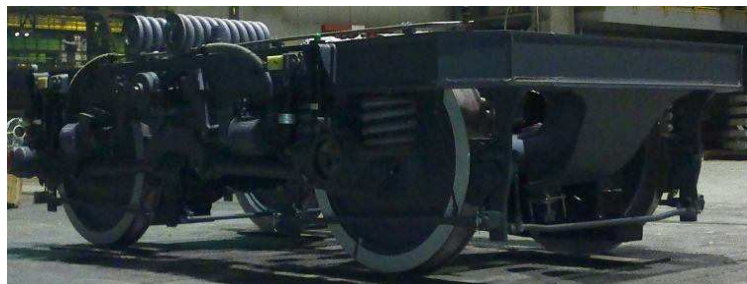
Fig. 6. The scheme of body connection with the bogie of the electric locomotive 2ES6 series "Sinara": 1 – inclined rod, 2 – body support of the type "flexi coil", 3 – vertical stop, 4 – vertical hydraulic damper
