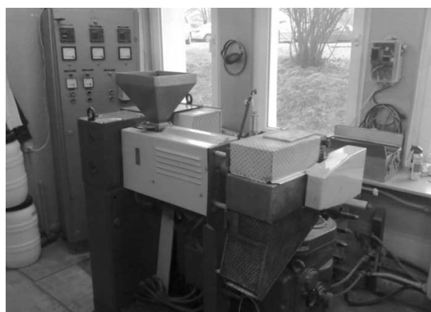
Fig. 1. Single screw extrusion-cooker TS-45 with L/D = 16 made by Z.M.Ch. Metalchem
