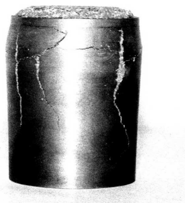
Fig. 2. Destruction of the chamber during densification ( p_k – approx. 145 MPa)
