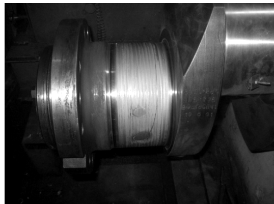
Fig. 4. Hardened crankshaft radical necks
