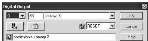
Fig. 3. Defining of the output signal for the control of the valve
