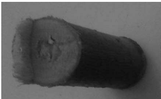
Fig. 6. The break in an almost totally cut sample
