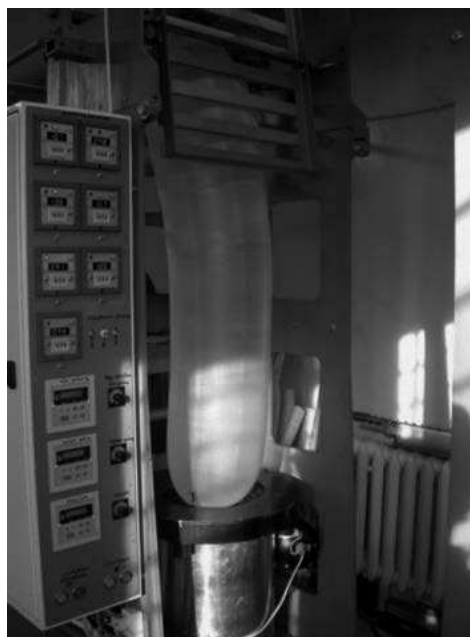
Fig. 1. The blowing of biodegradable TPS film in DFPE laboratory [5]
