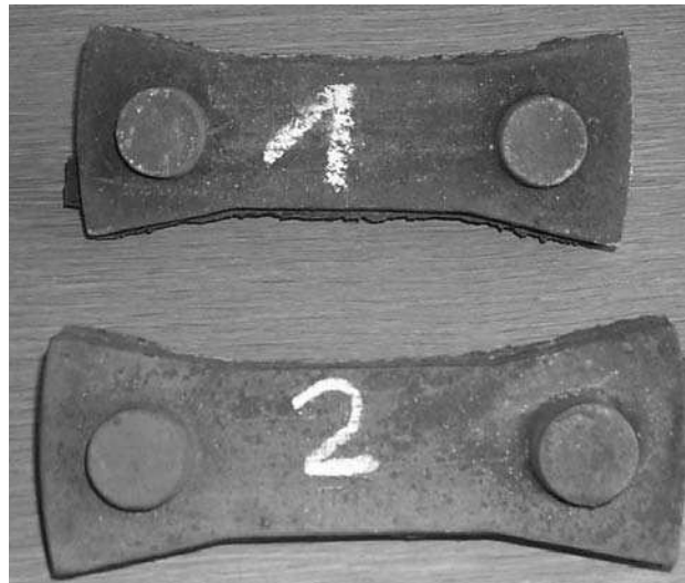
Fig. 4. Photographs of rams after de-gating
