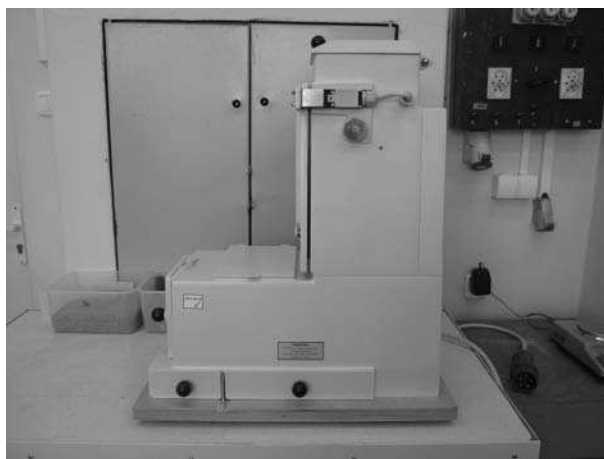
Fig. 1. Laboratory mill Quadrumat Junior
