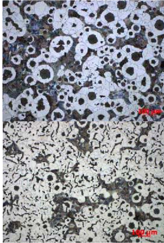
Fig. 1. Cast iron with flake graphite, spheroidal graphite and vermicular graphite
