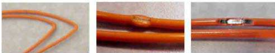
Fig. 4. Typical failures of fibre optic cables: bending, damage of sheath, damage of fibre [11]
