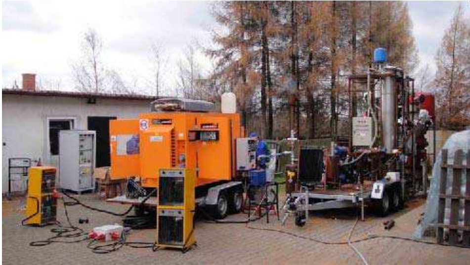
Fig. 1. The generating set connected to the gasification installation during the indication of the double-fuel engine [3]
