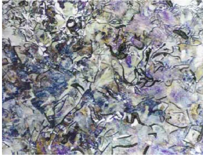
Fig. 4. An example of the structure of the tested grey cast iron
