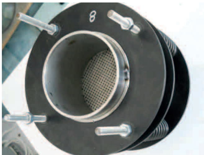
Fig. 1. Specially designed silo-stress simulator vessel
