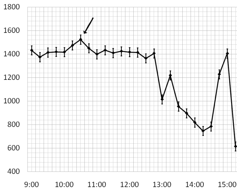
Fig. 2. Count rate of a vertical muon flux on November 6 th 1990
