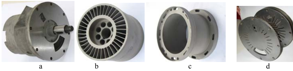
Fig. 2. Basic elements of construction of the experimental model of the CPE: a – stator; b – rotor; c – body; d – end face cover from the side of admission and rejection of compressing gas
