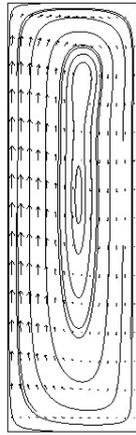
Fig. 2. Gas flow inside the OPC and isotherms (a cell 30 mm in diameter and 60 mm in length)
