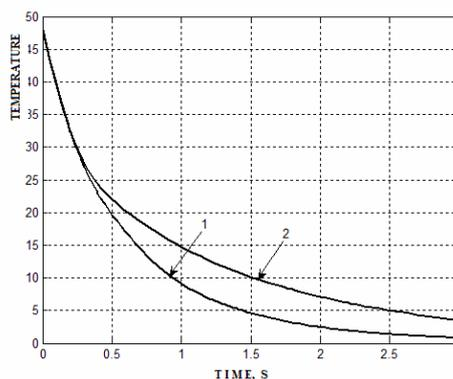
Fig. 3. Variation of the mean gas temperature in the cell (a cell 30 mm in diameter and 60 mm in length with regard for convection (1) and thermal conduction (2)
