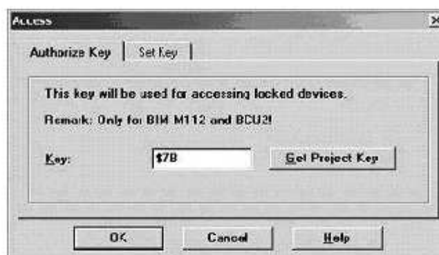
Fig. 9. Access authorization screen to the bus port in BIM M112 and BCU2 technology [KNX.org]
