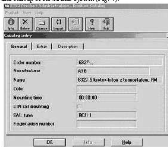
Fig. 7. Catalogue data screen for bus device [ETS manual, KNX.org, Petykiewicz P. 2001]
