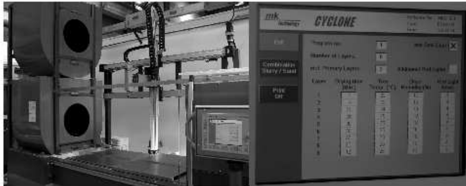
Fig. 6. The Cyclone II equipment and setting of process parameters
