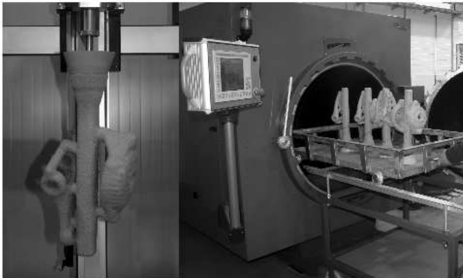
Fig 8. The ready ceramic layer mould placed in autoclave for melting out of wax
