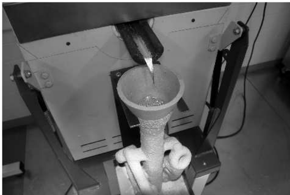
Fig.9. Pouring of mould with molten metal
