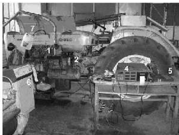
Fig. 2. The view of the test set-up: 1 – tested engine, 2 – angular velocity sensor, 3 – measurement interface, 4 – Technotest gas meter, 5 – control unit (notebook 486/33 MHz), 6 – Olivier smoke meter, 7 – changeable fuel tank
