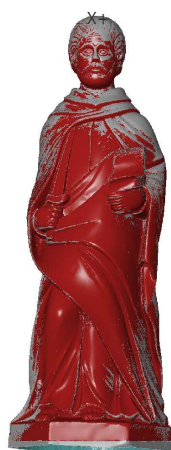
Fig. 15. Overlay of original statue (red) and BIS replica (in grey)
