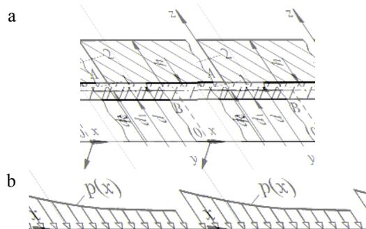
Fig. 1. The geometrical characteristics of connection with interference (a) and diagram of distribution of contact pressure (b)
