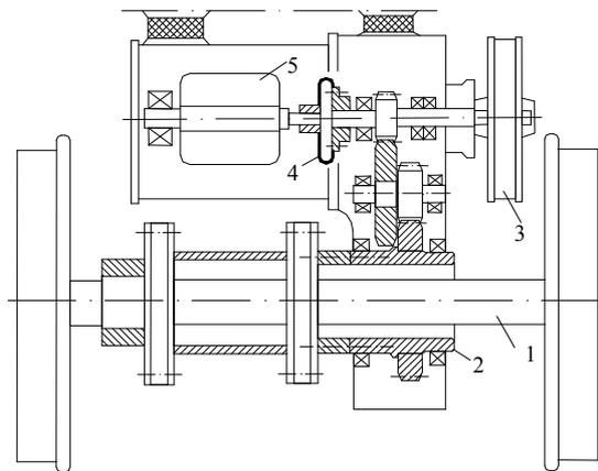
Fig. 2. Scheme of the generator drive in a passenger car: 1 – wheel axis; 2 - entrance the hollow shaft of gear ; 3 – conducting pulley belt drive; 4 – flexible coupling ; 5 – flywheel
