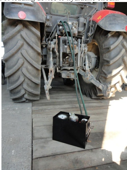
Fig. 2. The connection of the loading unit to hydraulic circuit of the tractor Zetor Proxima 7441
