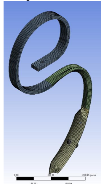
Fig. 15. FEM network of the 28x11 Tiller's sprocket developed manually [Own elaboration]
