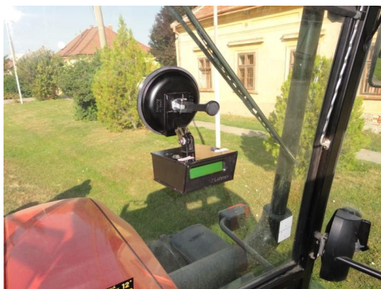
Fig. 1. The location of XL - Meter TM Pro Gamma on the windshield of the tractor Zetor Proxima 7441
