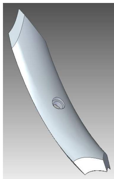
Fig. 6. Three-dimensional model of the tiller's sprocket tip following the option [Own elaboration]
