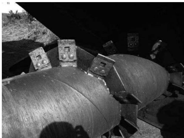
Fig. 2. Paddles on a rotor of the turning machine
